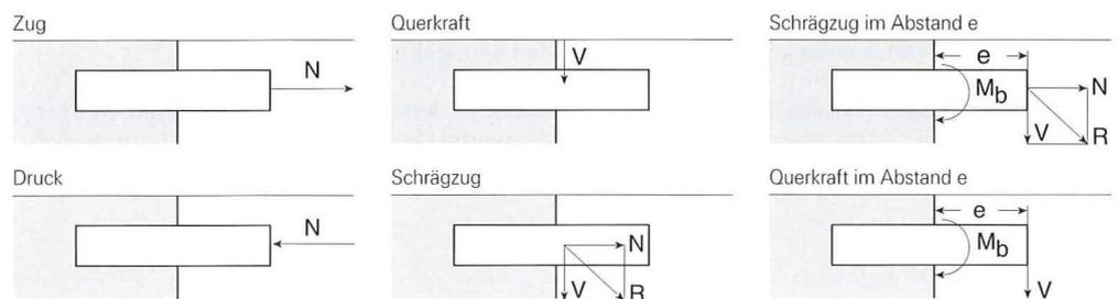
N = Normalkraft positiv/negativ, R = Resultierende, V = Querkraft,  $M_b$  = Biegemoment
