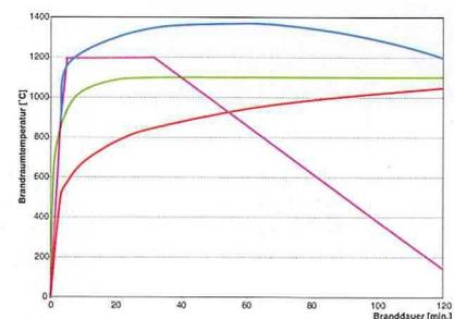
Temperaturkurven: — (ETK), — Hydrocarbon-Kurve, — RABT/ZTV-Tunnelkurve, — Rijkswaterstaat-Tunnelkurve
